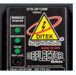
upon to protect certain devices, along with the severity of the applied power surges. That means that the shelf life of an SPD depends on consistent and regular visual inspections that are, concurrent with other maintenance. Some SPDs are designed with visual and/or audible indicators, such as LED lights and sounds, that alert you when a device is no longer functioning and needs to be replaced. Some SPDs also can provide remote notification of surge protection status to your systems.
