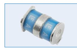
diverting the surge away from the device it is protecting. Once the surge has passed, the ions recombine to become gas molecules. While the GDT is ideal for protecting against extremely large surge events, it is less effective reacting to fast traveling and sudden surges.
