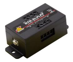
**DITEK's DTK-2LVLPF** is specifically designed to protect 24V Signaling Line Circuits (SLC) on fire alarm control panels. Its robust surge current rating and tight clamping performance helps to prevent induced surges from damaging sensitive control boards.
