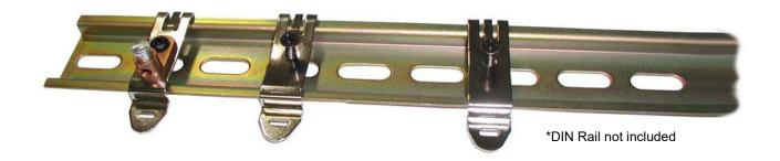
DITEK's DTK-DRK Series DIN Rail Mounting Kits allow integrators and installers to adapt a wide variety of DITEK surge protectors to easily mount on standard 35mm DIN Rails. Each kit includes screw-on adapter clips to easily mount various DITEK surge protectors onto DIN Rail flanges. A grounding lug provided with the DTK-DRK kit allows the surge protectors to ground directly to the rail.
