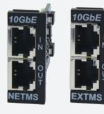
As an additional flexibility benefit, all enclosures are compatible with the DTK-NETMS and DTK-EXTMS Ethernet, PoE and PoE Extender protection modules if desired. These modules carry a robust 20kA per pair surge current rating, support data speeds up to 10GbE without signal degradation, and comply with IEEE Power over Ethernet standards.
